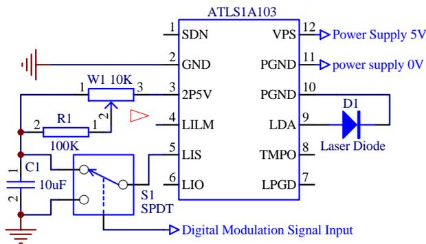
Figure 4 Low Noise Digital Modulation Circuit
