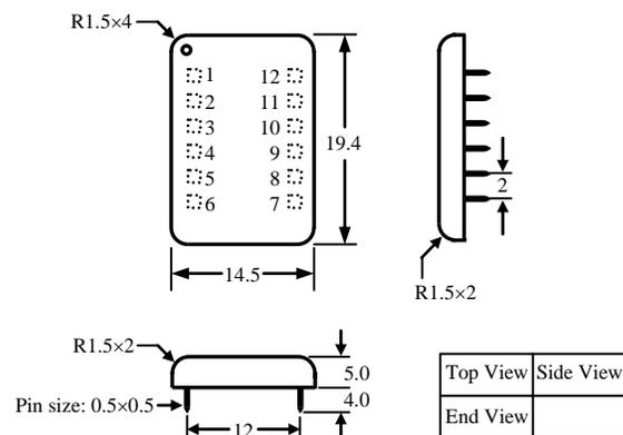
Figure 5 Dimensions of the DIP Package Controller
