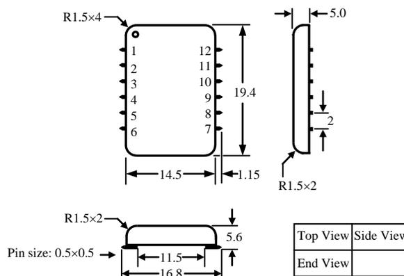
Figure 8 Dimensions of the SMT Package Controller
